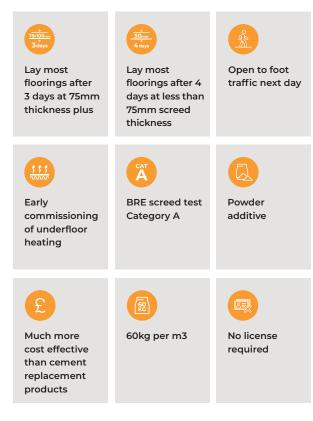
RonaScreed 4 Day Overlay powder additive is used to quickly reduce the level of retained moisture within site batched screeds. This allows floor coverings to be laid much sooner than with conventional screeds. Rapid strength gain permits early access by following trades.
