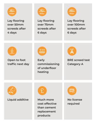
RonaScreed FastDry Prompt is a fast drying additive for site batched screeds used to quickly reduce the level of retained moisture within the screed. This allows floor coverings to be laid over the screed much sooner than with conventional screeds. RonaScreed FastDry Prompt gains strength quickly, permitting early access by following trades.
